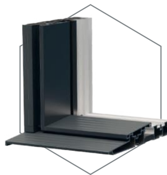
Low Threshold with Ramp (25mm high) tested to the requirements of Part M. Only available on double track designs
